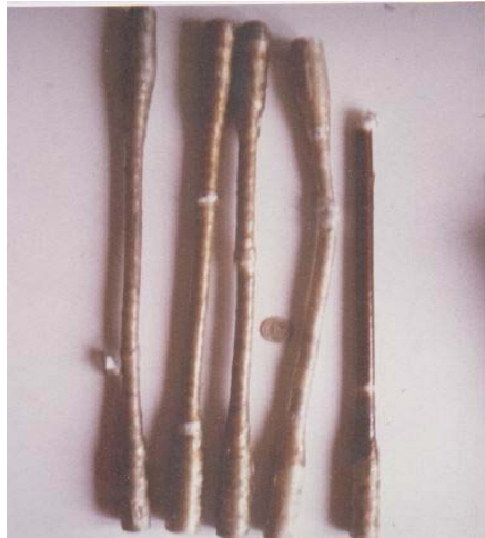
The First Laboratory Samples of Composite torsion beams tested in 1983
