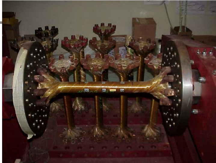
Torsion beam 60 mm diameter 600 mm long; ultimate torque 280 000 N*meter @ 60 ° of torsion Up to 1992
